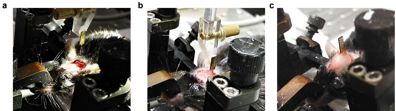
Figure S13. Experimental procedure of implanting the flexible probe. a) expose the mouse skull and a small hole is made by a drill; b) implant the microprobe into VTA, and apply dental cement fix the probe; c) release the holder after dental cement is dry.
